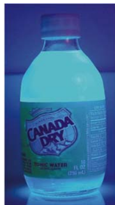
■ Figure 30.8 Tonic water is clear under normal light, but vividly fluorescent under ultraviolet light, due to the presence of the quinine used as a flavoring.
